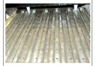
The horizontal evaporator and water distribution system are unique to the Hoshizaki IM series. The IM-500 makes ice on a horizontal evaporator and uses R-404a refrigerant.
